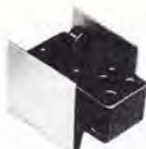
PP4616 Clip-in fused terminal block assembly with 3A fuse. Primary use for Popular Pack fitting when used on Trakline. Encroaches on centre entry on 2ft. 20W twin only. Not for use in 6ft. fittings. These contain a fuse as standard practice. Standard quantity 5 per pack.
