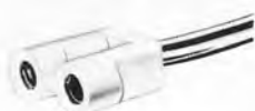
AME M6064/12/Loop Starter Socket White PVC moulding enclosing starter switch contacts crimped to 12in loop 14/0076 white PVC cable which can be cut at a point to suit wiring layout. Current item for 2ft fittings and for earlier Popular Pack fittings in other sizes.
