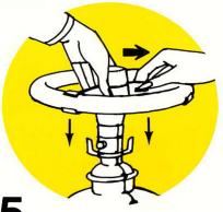
Line up raised section on ADAPTER with groove in SATELLITE. Make sure groove is pointed downward to allow access of raised section. With tan plug pulled outward (away from inner ring), place SATELLITE onto ADAPTER.
