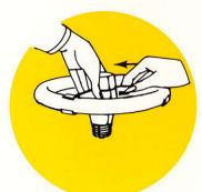
4 Grip CIRCLITE as shown in the illustration and screw into ceiling socket. Tighten gently. (Do not install by turning the glass portion of the SATELLITE.)
