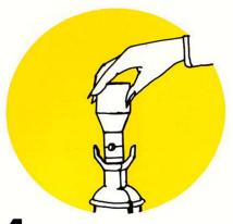
Screw ADAPTER into lamp socket and gently tighten as you would a household light bulb.
