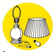
Turn lamp off. Unplug lamp from wall socket. Remove shade and light bulb.
