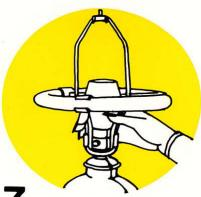
Replace harp by sliding ends down between the SATELLITE. Carefully squeeze both harp ends together, place in position and lower retaining bells.
