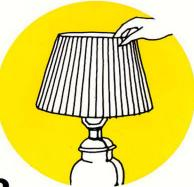
Replace shade and plug portable lamp into wall socket. When turning portable lamp on, flickering may occur before starting. This is common with fluorescent tubes.
