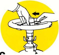
Push up and slide tan plug completely forward toward center of ring to lock SATELLITE and make electrical connection to the ADAPTER.
