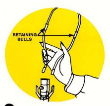
Remove harp. To remove, raise retaining bells, squeeze harp ends together and lift out.
