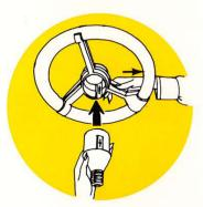
**3** Push up and slide tan plug *completely forward* toward center of ring to lock SATELLITE and make electrical connection to the ADAPTER.
