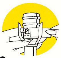
Apply enclosed tape to provide added strength to the socket as illustrated.
