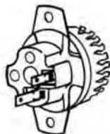
G.L 1042/HV for lamp voltages over 21-5V
